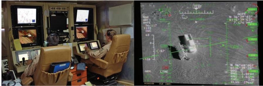
Fig. 8. Command center of a military UAV's operator. (Adapted from [69])
