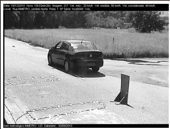
Figure 7. Photographic record generated by the instrument, configured with sensitivity level of 0.01%, for the test vehicle passing at 100 cm from the sensor.
