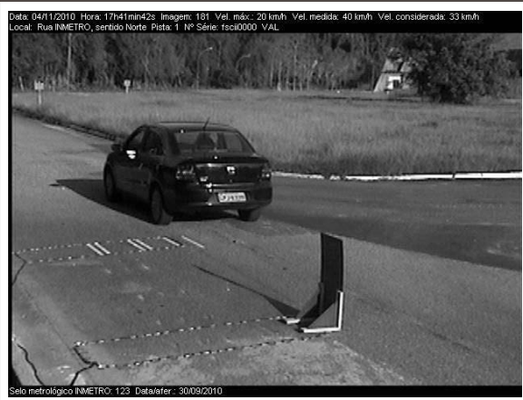
Figure 5. Photographic record generated by the instrument, configured with sensitivity level of 0.04%, for the test vehicle passing at 20 cm from the sensor.
