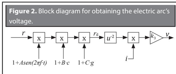
In the figure above,  $c$  is a low-frequency chaotic signal generated by Chua's oscillator (Kennedy, 1993) and  $g$  is a random signal with Gaussian probability distribution (Manchur, 1992). The constants  $A, B$ , and  $C$  represent the range modulation indices for the three modulating signals. Once  $r_d$ , the electric arc's dynamic voltage by phase, is obtained, it is determined by the following equation:
