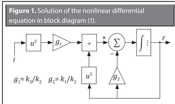
In the three-phase arc furnace model, we must obtain a respective value of  $r$  for each line current. Once  $r$  has been determined (by phase), the second part of the model determines the electric arc's dynamic voltage. To do so, we first modulate the range of  $r$  with the three signals, that is, the sinusoidal signal, the chaotic signal, and the random signal with Gaussian distribution. **Figure 2** shows the implementation of the model's second phase in a block diagram.
