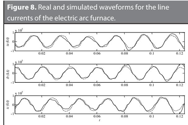
In the figure above, we can see that the simulated currents follow the real currents with a high degree of precision in some cycles and that in the remaining cycles, the currents move apart at the positive and negative extremes. The percentage errors obtained for the electric arc currents were 0.88% for phase *a*, 0.08% for phase *b*, and 4.1% for phase *c*.
