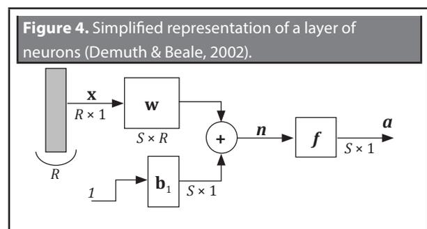
Due to the total connection of input signals  $x_i$  with the respective neurons, the number of synaptic weights for each neuron is equal (in dimension), and it is therefore possible to group said weights in a  $\mathbf{W}$  matrix, called the synaptic weights matrix.
