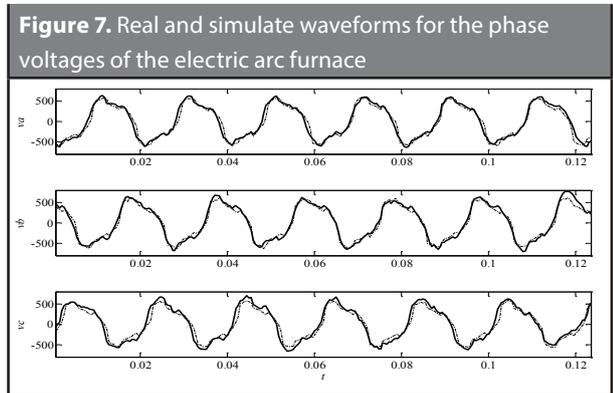
In this figure, we can see that the arc furnace model captures the non-linear nature of the real voltages and also that the values of the parameter vector components obtained with the algorithm allow us to obtain voltage levels similar to real levels. The percentage error obtained for the phase voltages was 1.17% for phase *a*, 2.79% for phase *b*, and 2.94% for phase *c*.
