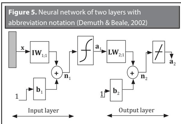
In accordance with the figure above, the mathematical model of the output function  $a_2$  of the neural network is described by the following equation:
