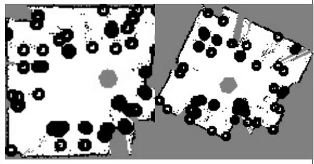
**Fig 13.** Feature points extracted by Shi-Tomasi Detector in images generated by SLAM algorithm.
