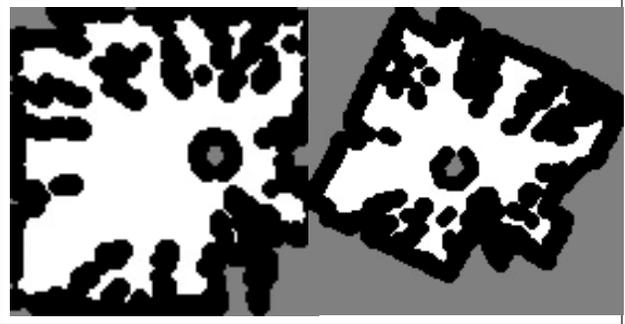
**Fig 15.** Feature points extracted by our corner detector technique in images generated by SLAM algorithm.
