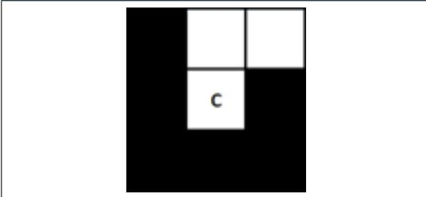
With these simple rules, the algorithm designed for feature extraction by detecting corners, makes a fast search by reducing the workspace since it discards pixels with irrelevant information or pixels with a low value on grayscale. However, discarded pixels are analyzed in other iterations if they are near to a real corner, so it is important because discarded pixel can provide us information that helps to define the appearance of a corner in the image.
