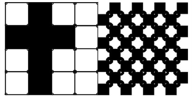
**Fig 9.** Feature points extracted by Shi-Tomasi Detector. As it was expected, this technique achieved same results of the Harris Corner detector, because Shi-Tomasi is based on Harris.
