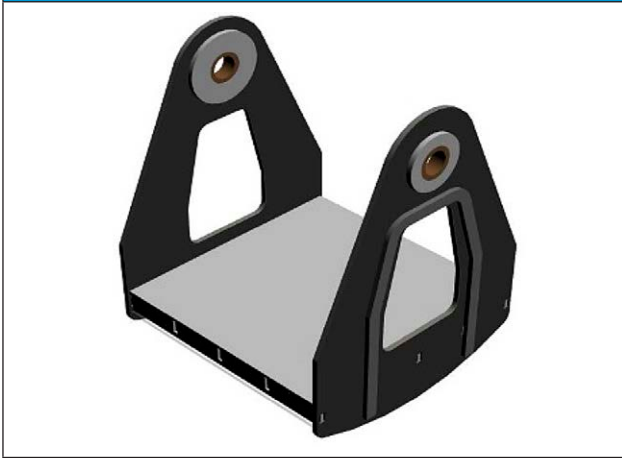
Fig. 7. Geotechnical centrifuge swing. Source: Authors
